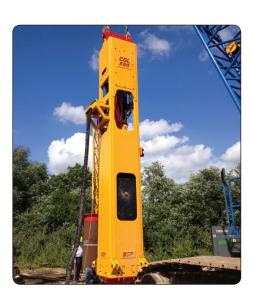
**Above:** Hammers shown in leader mounted operation. Crane suspended option also available.
